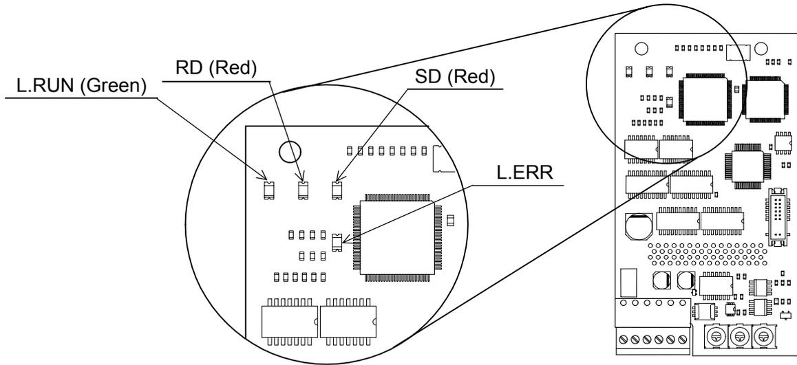
Note: For details of LED display, refer to 7.2 *CC-Link Interface Card LED Display*.
