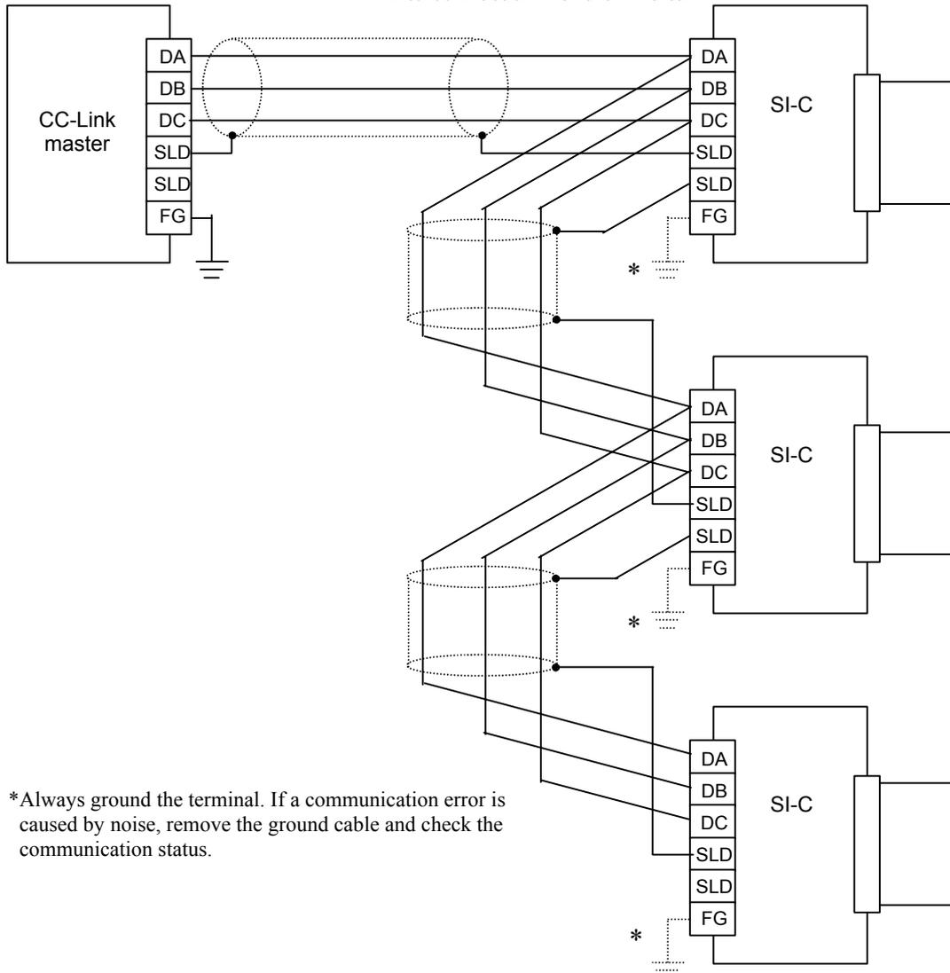
\*Always ground the terminal. If a communication error is caused by noise, remove the ground cable and check the communication status.
